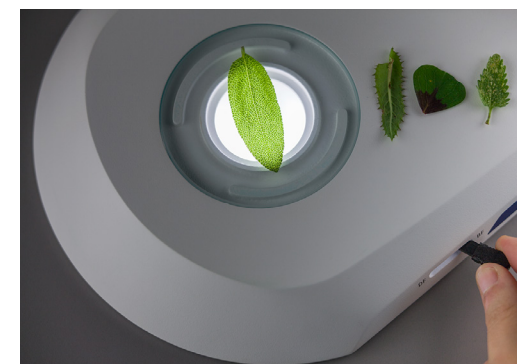
Use the flat transmitted light unit to contrast colored transparent specimens in bright- and darkfield. Add polarizer/analyzer equipment to observe, for example, birefringent crystals or tensions in glass or plastics.
