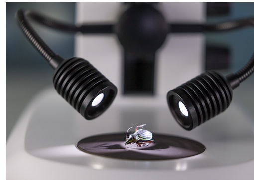
For sample preparations in reflected light, the double spot illumination with self-carrying goosenecks is optimal. It creates half-shadow effects that lead to a good 3D impression without overly dark shadows. During dissections the specimen stays illuminated even if the manipulating hand covers one of the spots.
