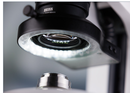
The shadow-free ringlight features four different segment modes: full-, half- and quarter-circle and 2-opposite quarter-circle. Set the segment illumination, then turn the light direction manually in 90° steps to quickly inspect for scratches, defects or residues without moving your specimen. Or use auto rotating mode to get a spatial impression of the object surface just by changing shadows.
