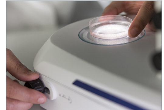
The tiltable and shiftable mirror features brightfield, one-sided darkfield and oblique light – plus polarization contrast as an option. Rotate to frosted and plain mirror side, then decide between crisp and diffuse brightfield contrast.
