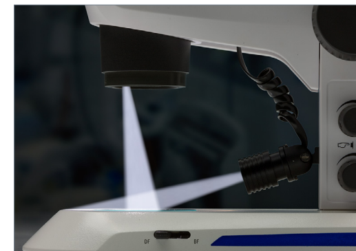
Easily switch between vertical illumination, oblique spot or mixed light by the push of a button – and adjust their intensities.
