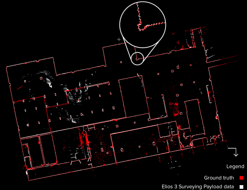
Overlap of a Surveying Payload 3D point cloud with the ground truth used to assess the LiDAR accuracy
