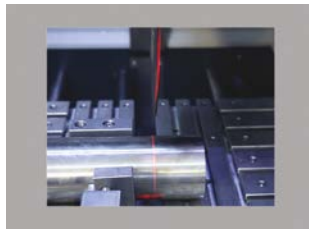
Laser alignment unit (for MA & AA models) (To be ordered simultaneously together with the machine order)
