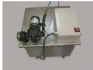
Recirculating Coolant System
