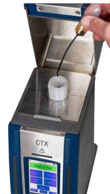
Bruker's light-weight, portable CTX™ 800/600 models or the handheld S1 TITAN™ 600/800 models are optimized with the Metals in Oil Calibration for ready-to-go testing. The CTX is safety interlocked and self-contained. A fitted backpack carry case for easy transport up ladders is available. The S1 TITAN is an open-beam handheld which provides the additional benefit of being agile enough for in-situ measurements. It can be used for liquids with an available desk top stand.
