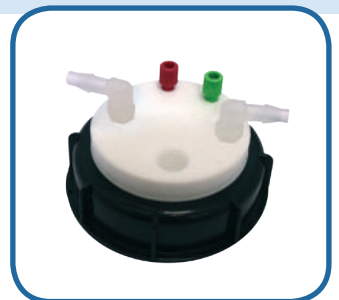
SW90-2-C-2L : 2 entries 1/8", a charcoal cartridge emplacement and 2 threaded barbed fittings
