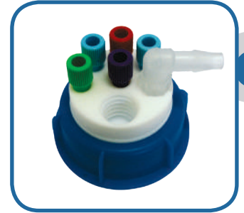
SWB-5-C-1L : 5 entries 1/8", 1 threaded barbed fitting and charcoal cartridge emplacement
